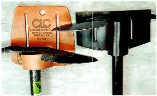
Spade-picks in sheaths. The one on the left is a standard sheath that is designed to hold a hammer (Custom LeatherCraft, Model #426). The spade-pick sheath on the right is one I built myself.
